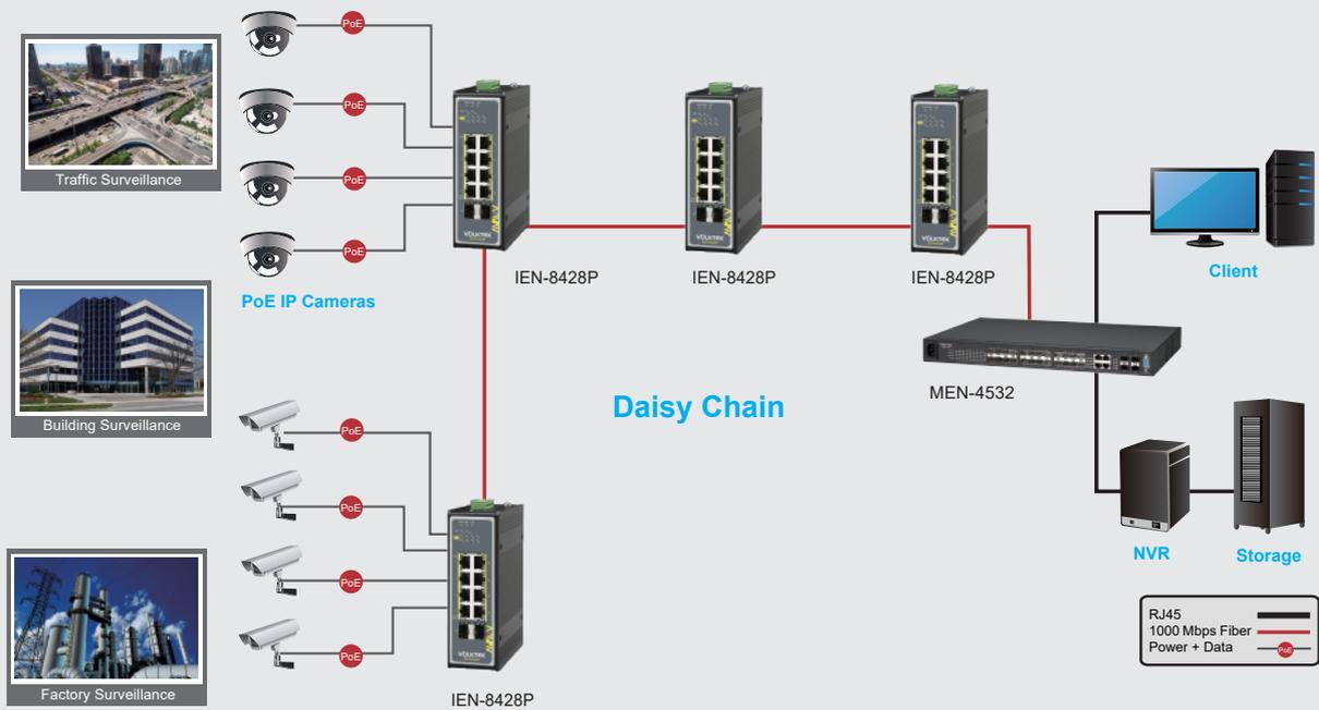
The IEN-8428P is compatible with 10/100/1000Mbps through RJ45 transceivers to guarantee a strong, stable connection of Ethernet, Fast Ethernet or Gigabit Ethernet, providing flexible deployment options to satisfy industrial networking requirements.
